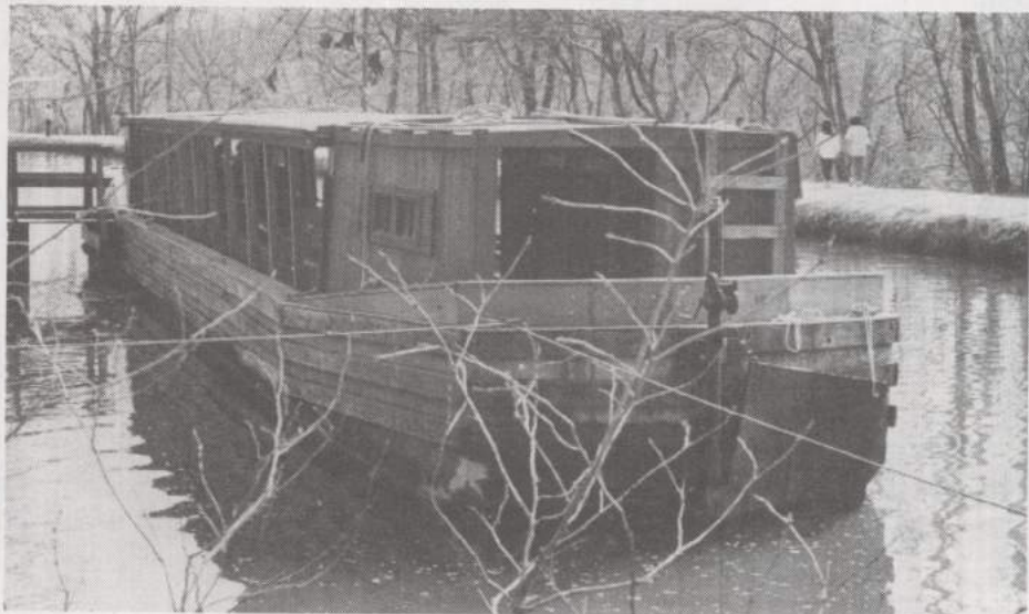
Barges such as this were pulled by mules along the towpath of the C&O Canal, bringing freight of many kinds to and from Cumberland and Georgetown, D.C.
